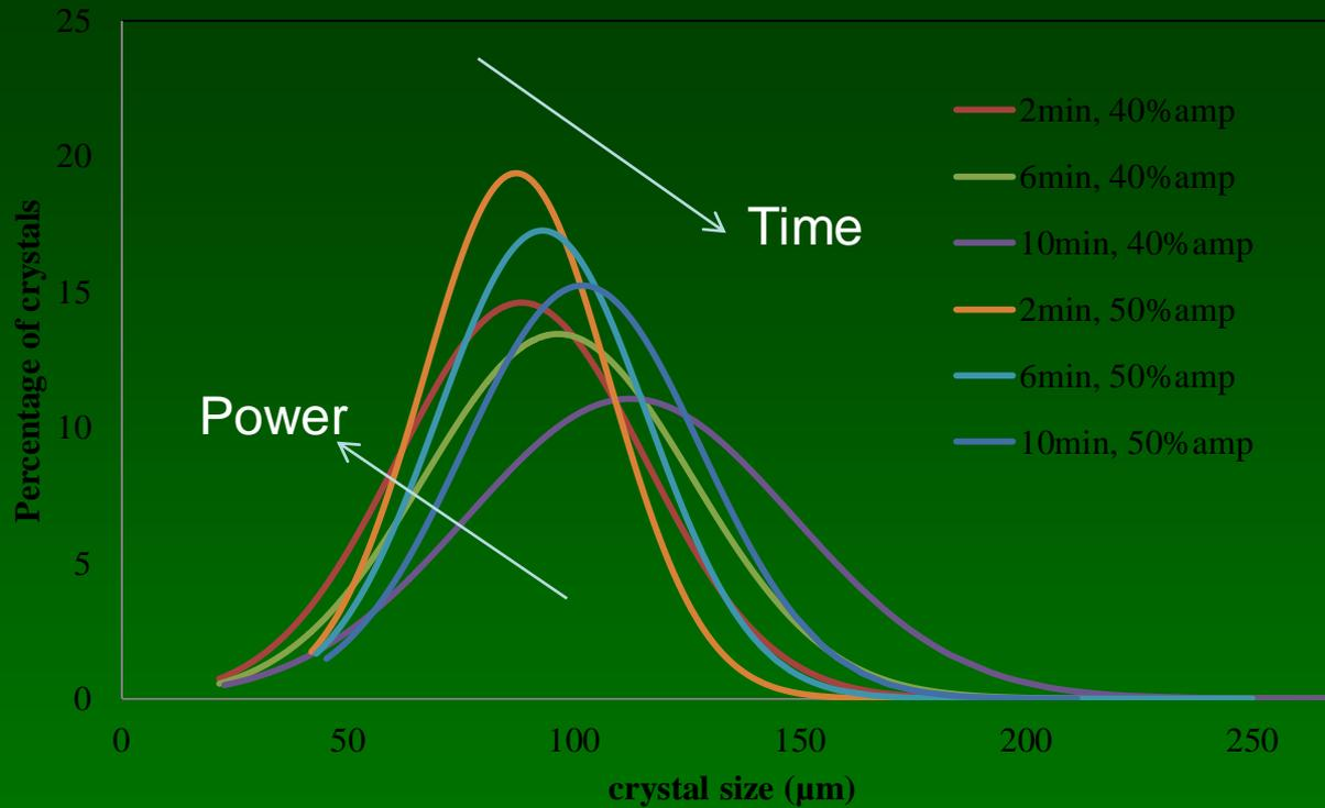
Increase in crystal size with respect to time at 40% and 50% amp of ultrasound at 0.018ml/s of addition rate.
