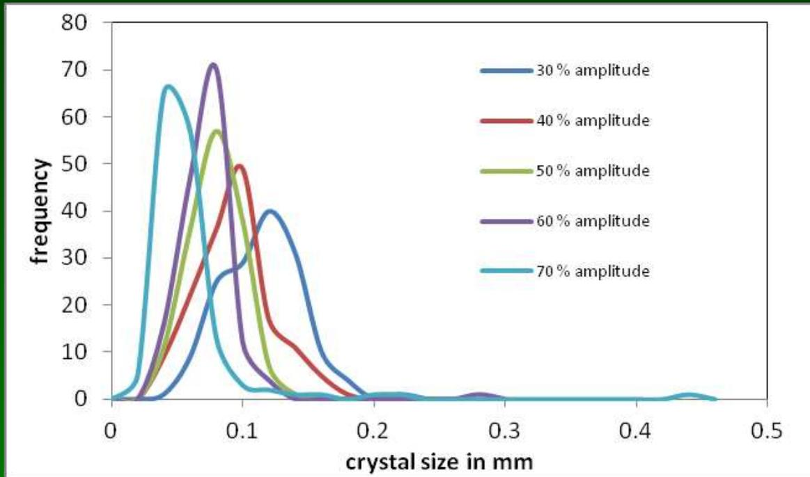
Effect of ultrasonic power on crystal size distribution of dimethyl sulfone
