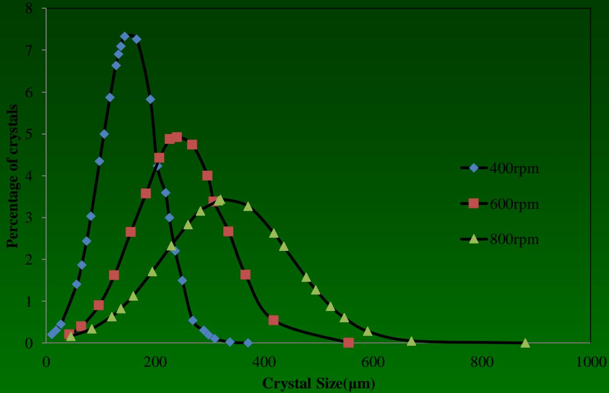
Effect of agitation rate on the crystal size of benzoic acid at flow rate of 0.018ml/s
