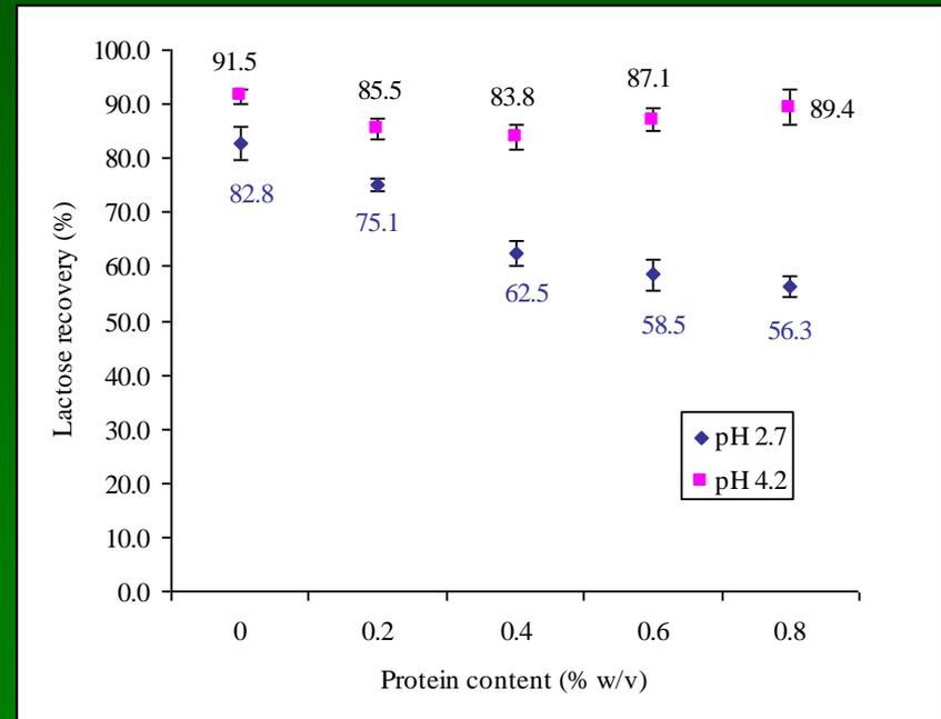
Effect of inhibition in crystallization due to protein > in solution with low lactose concentration
