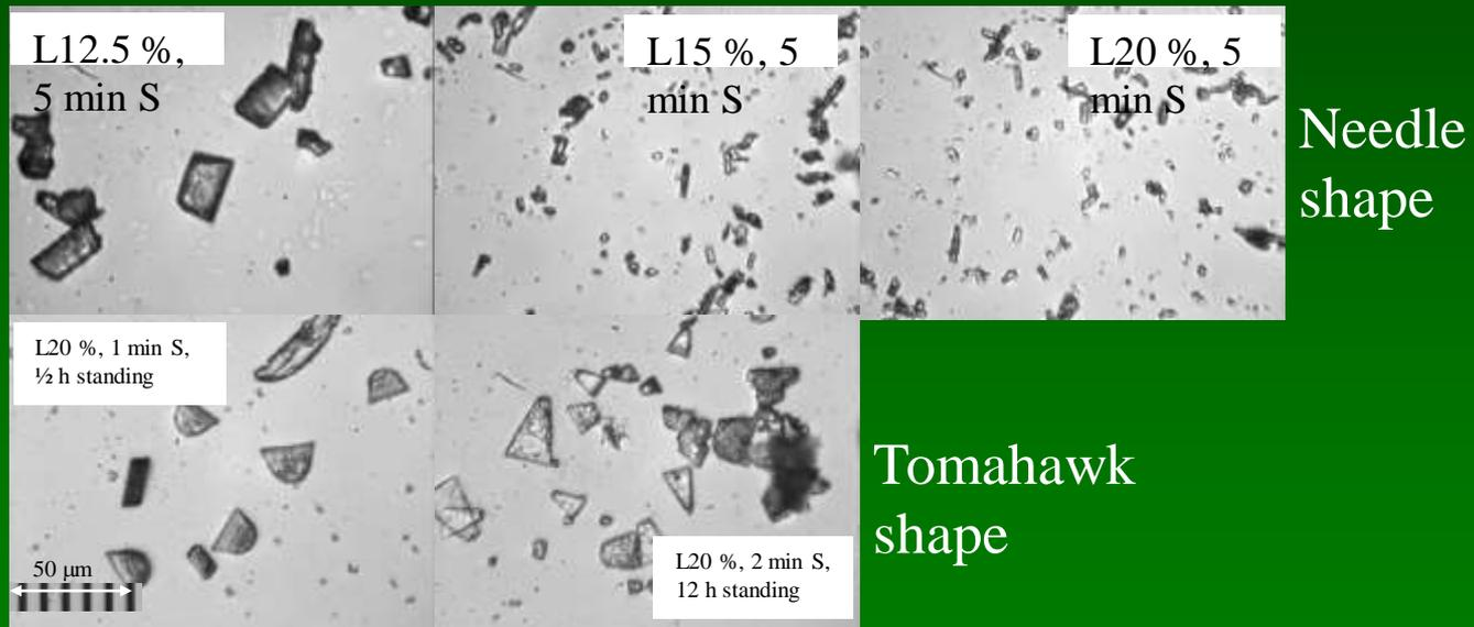
Crystals observed under Leica Gallen microscope (40 X objective)
