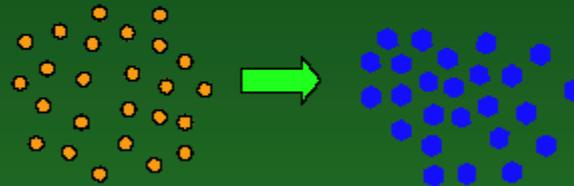
Using insonation to only initiate nucleation allows larger crystals to grow
