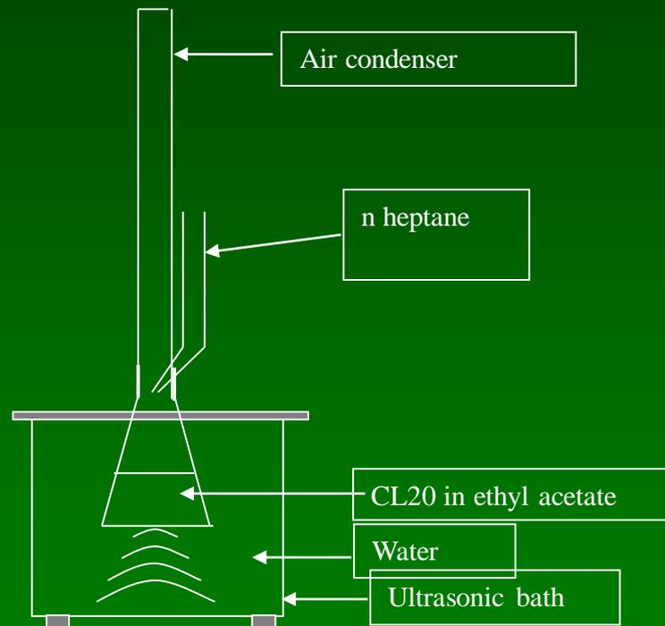
Schematic representation of the Experimental set up
